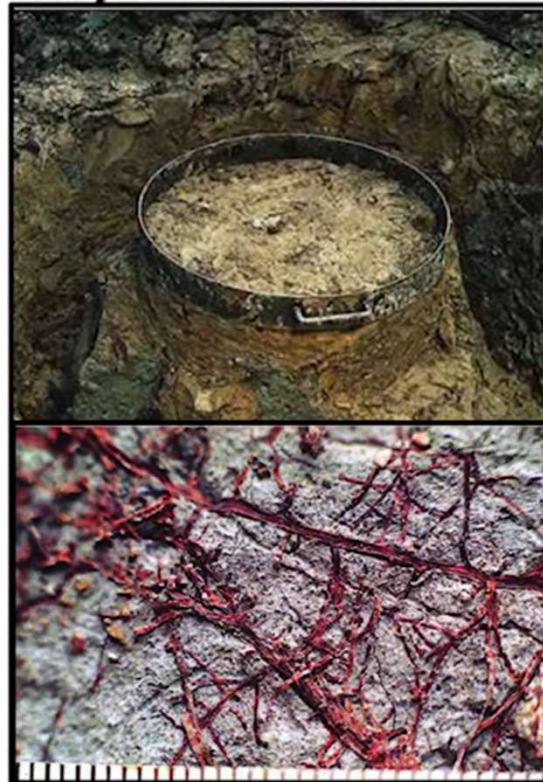
Root Imprints on Gray Fracture Surface
