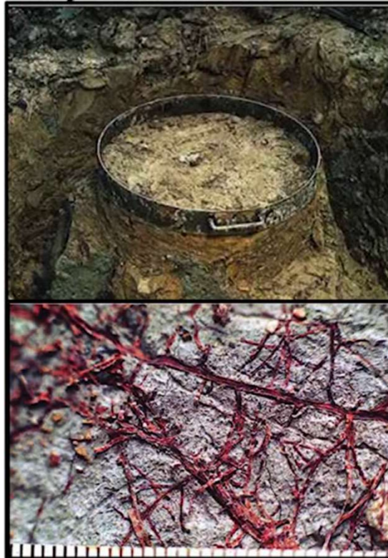
Root Imprints on Gray Fracture Surface
