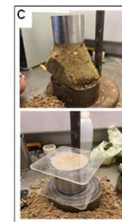
Intact cores of matrix hydraulic tests
